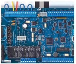
Master/Member network using HeatNet protocol, or as a member in a system for up to 16 boilers. HeatNet provides a higher level of control precision, repeatability and feedback with digital communications control, featuring four (4) temperature sensor inputs: outside air, supply (outlet) temperature, return (inlet) temperature and header temperature. HeatNet is fully compatible with Modbus Building Management System (BMS) protocol.
